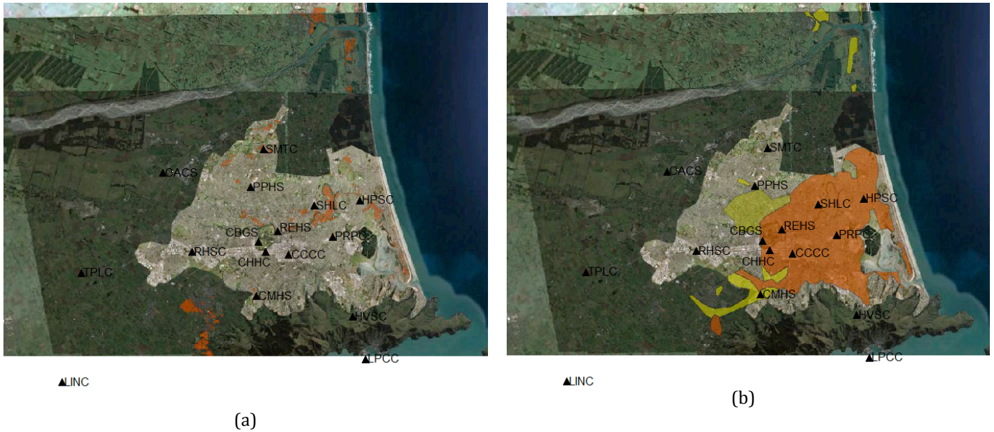
Fig. 3. Liquefaction distribution in the Christchurch area during the (a) 2010 Darfield earthquake and (b) 2011 Christchurch earthquake. Brown color areas are the severe damage areas.
