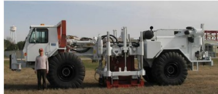
b. Low-frequency, two-axis shaker called Liquidator
