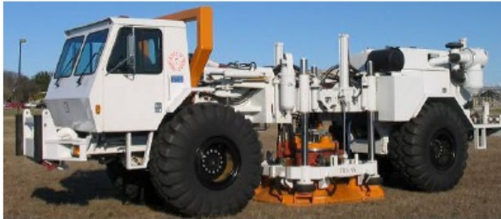
a. High-force, three-axis shaker called T-Rex
