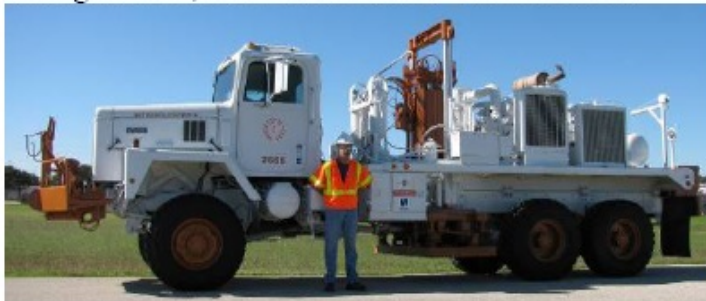
c. Single-axis, vertical shaker called Raptor
