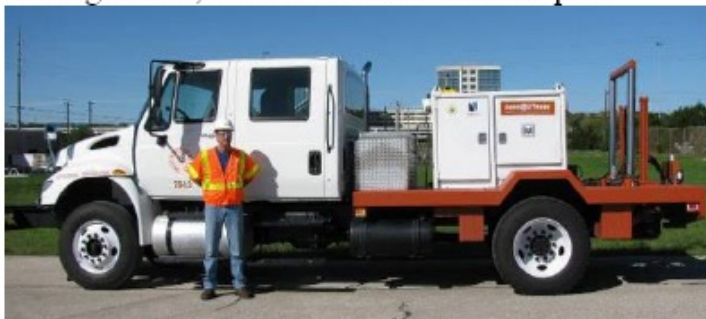
e. Urban, three-axis shaker called Thumper
