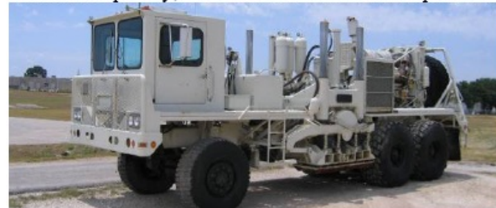
d. Single-axis, horizontal shaker called Rattler
