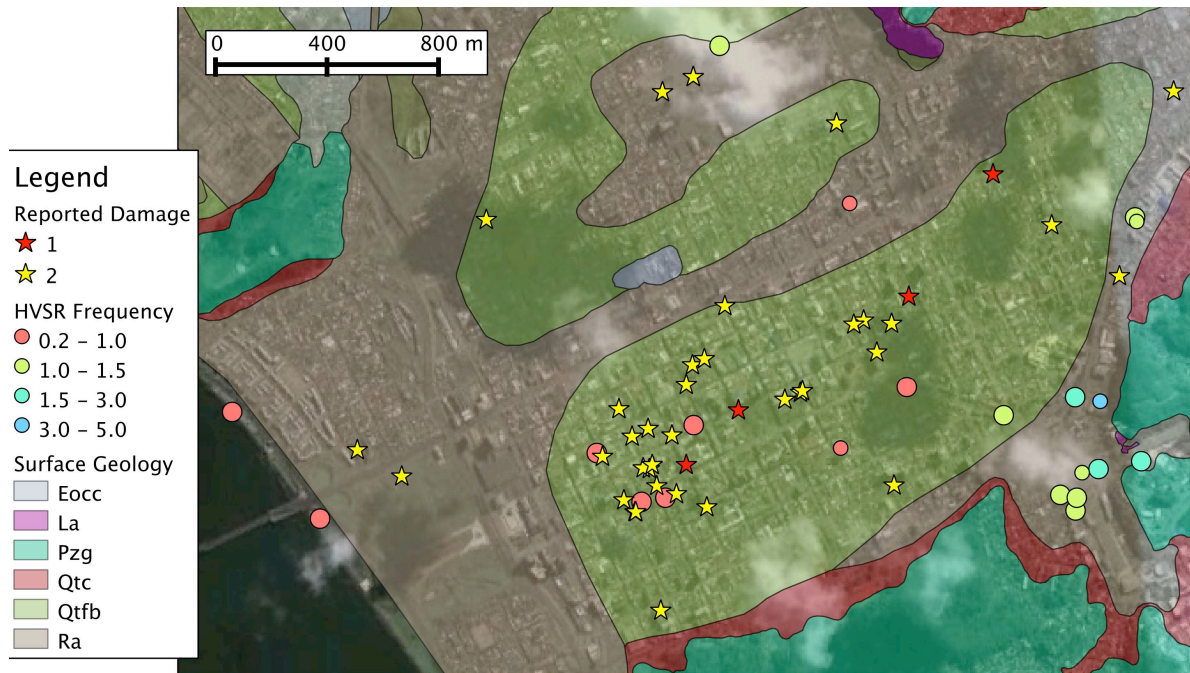
Fig. 4. Aerial photograph with the surface geology found in Concepción (modified from Galli, 1967), the corresponding legend is shown to the left. The stars mark the location of severely damage buildings after the Maule 2010 earthquake (see text for details). Circles show the location of a microtremors measurement, with the color proportional to the predominant frequency (see legend) and the size to the HVSF amplitude.
